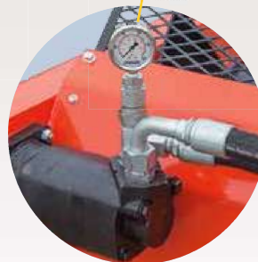
Visible hydraulic pressure gauge
